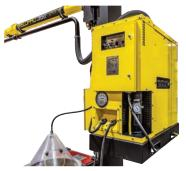
Integrated Fume Extraction System that moves with the welding arm. (shown column mounted)
