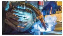
The extraction unit and fume extraction gun move with the operator.
