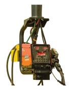
capable of controlling the power supply remotely. Boom/Arm controls are placed within arm's reach of the operator increasing their productivity and safety.
