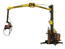
WeldPro 360 LRW-18P MIG Welding **Booms** reduce or eliminate non-arc time welding-related tasks, shop floor clutter, and employee safety issues. This arm provides complete coverage anywhere within a 56' diameter semi-circular welding zone. The welding arm's main pivot assembly mounts to your existing building column, freestanding column or the optional mobile base and column
