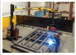
This eliminates wasted time walking back and forth to the welder to change weld settings. Welding wire conduit liner, power cable, gas and air hoses are all contained within the tubular arms eliminating safety hazards and shop floor clutter. This makes for a neat, clean, organized shop.
